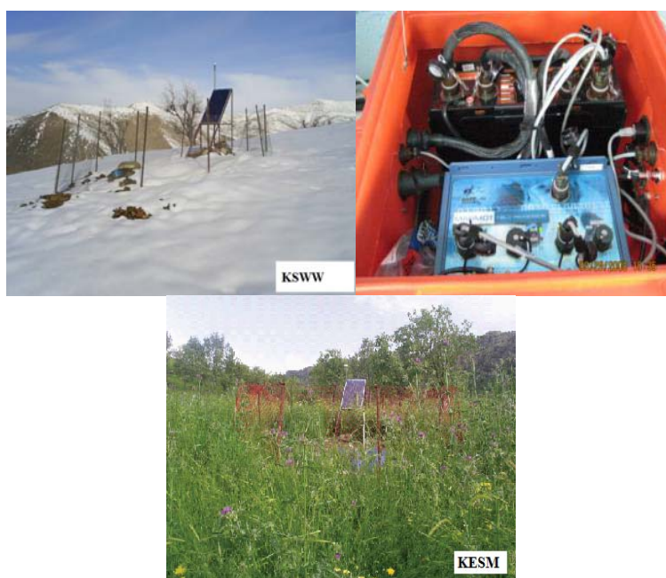
Fig.1: Shows two of the NISN stations, solar panels, GPS antennae with the STS-2 seismometer, Q330 digitizer and baler data storage.
